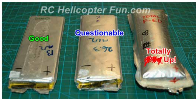
Levels of LiPo puffing from none on the left, to drum tight on the right.
