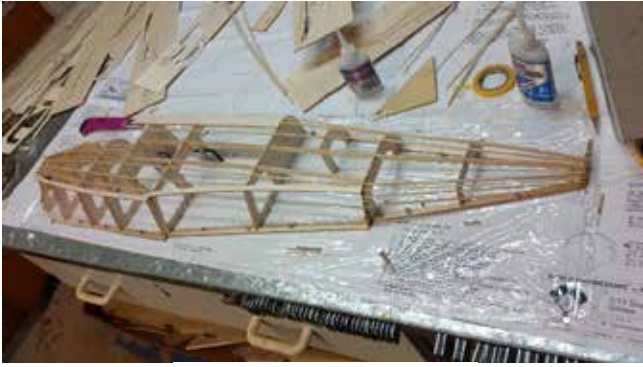
Getting some stringers laid in
