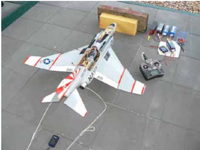
Static thrust and current/wattage tests using various batteries
