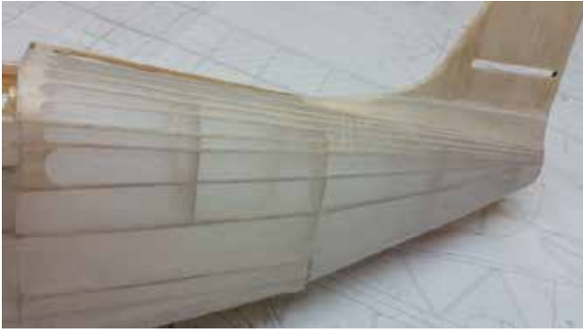
Each side covered in one piece to centre stinger top and bottom
