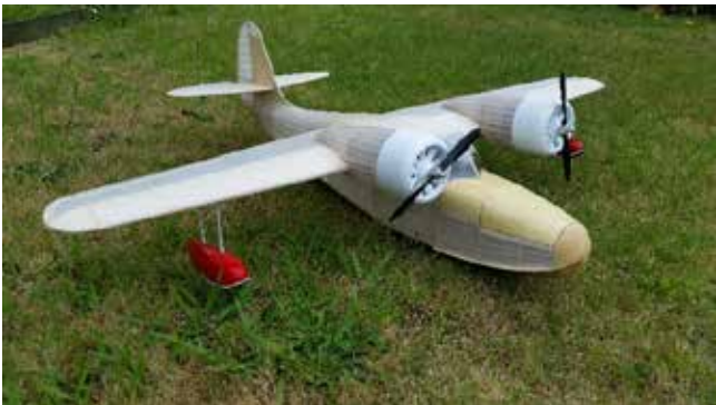
Edge trimmed and sealed, deliberately leaving an overlap. Can you see where I slipped with the scalpel and had to patch it? :-)
