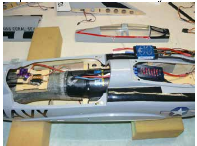
130 Amp OPTO/ESC replacement
