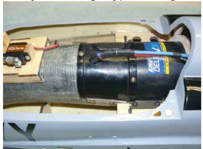
Duct cover secured with some ply and self-tapper screws.
