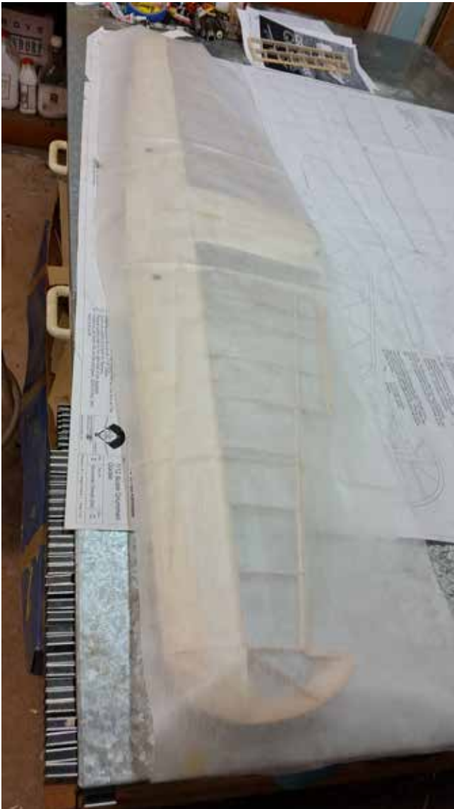
Sheet of Polyspan laid over wing
