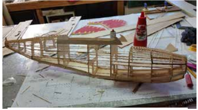
We have a fuselage. Red sauce bottle has Titebond glue in it
