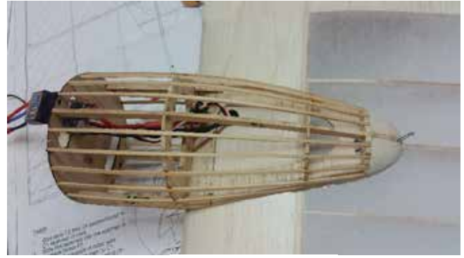
Nacelle glued in place
