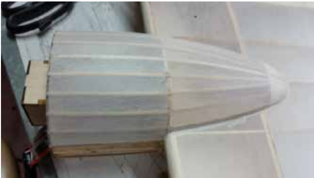
Edge trimmed and sealed, deliberately leaving an overlap. Can you see where I slipped with the scalpel and had to patch it? :-)
