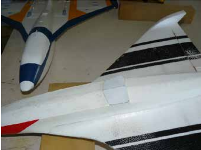
A view of the current skid kicker on my small HK Skipper – works like magic
