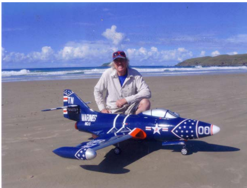
Joseph Frost (Bananacoast Radio Control Flyers) with his F9F Panther EDF. 3.5kg of batteries (12S) provide 9.3kW drawing up to 220Amps
