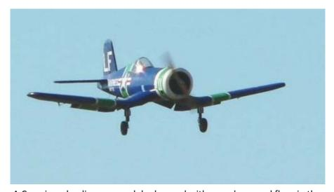
A Corsair on landing approach looks good with gear down and flaps in the landing position. This plane is powered by a 62cc gas engine.
