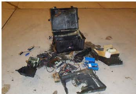
Figure 1: Fire-damaged bag and contents
