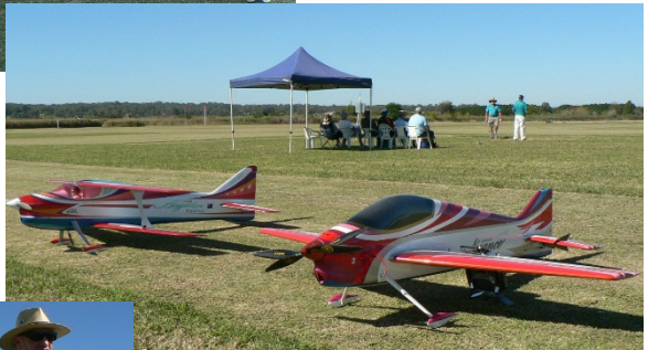
F3A State of the Art equipment with the newest plane belonging to Matthew Bailey a YS 175 CDI powered Biplane, and also shown is and Gavin Dark's Electric Monoplane with contra-rotating propellers. Mathew Bailey is the Nationals Champion in F3A for 2013, and is representing Australia at the next World Championships in South Africa in August this year.
