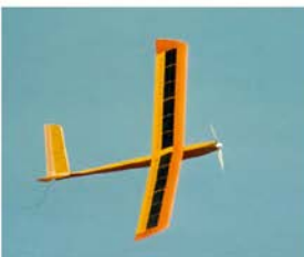
Solar Uhu of Graupner 1991. Kit of a solar powered model aircraft
