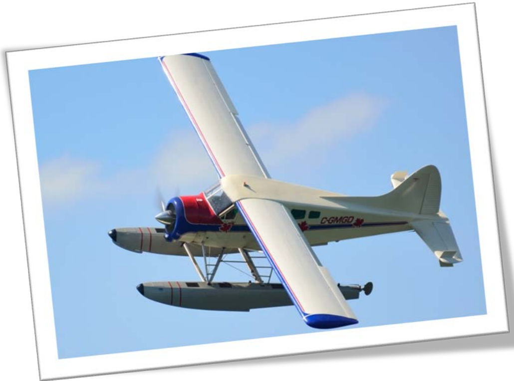
120" span deHavilland Beaver, 3W 56 twin for power, 21kg, Spectrum Radio
