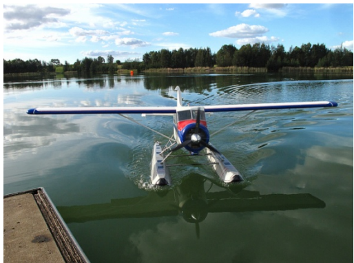
Aranka Nolan's 120" span de Havilland Beaver, 3W 56 twin for power, 21kg, Spectrum Radio
