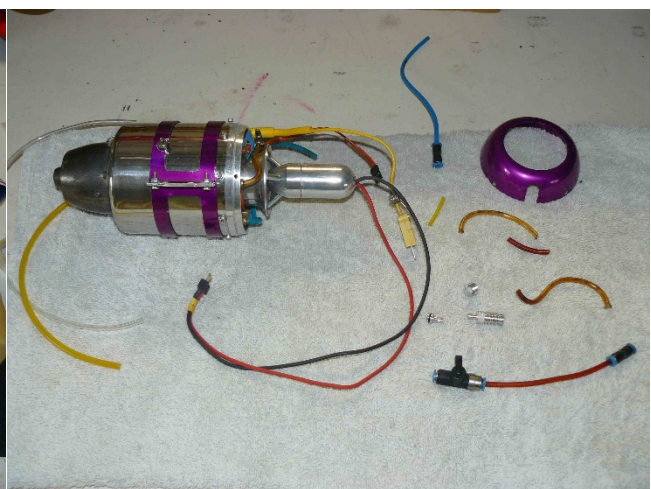
Crumbled fuel and gas lines
