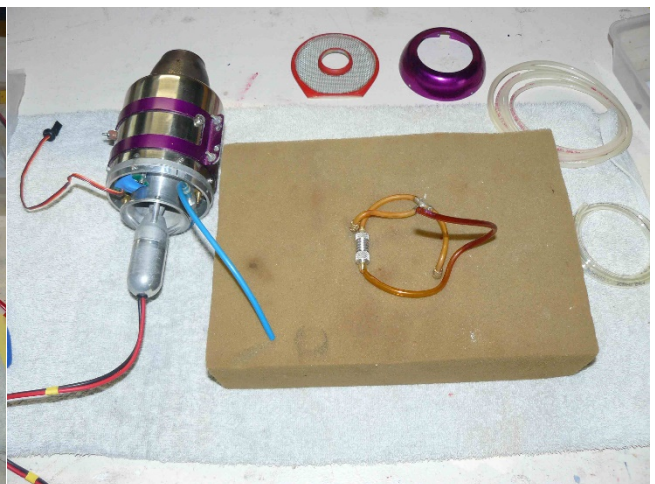
Stiff fuel lines after years of use
