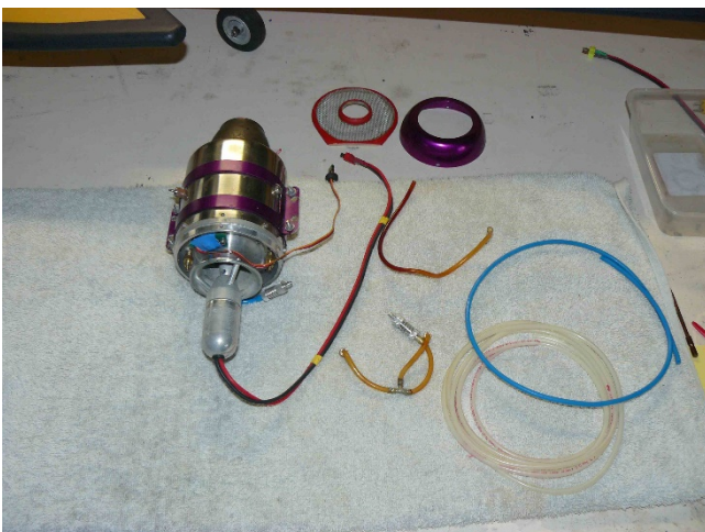
Gas line partly broken over the filter's nipple and at the rubber grommet exiting point, also found all fuel lines in very poor/brittle state
