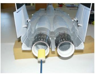
Further improvements were made to the rather inefficient twin inlet/outlet ducts for a single power EDF by smoothing, filling-up all the imperfections inside and a final sealing and gloss finish. The stock 4.5mm straight cut trailing edges
