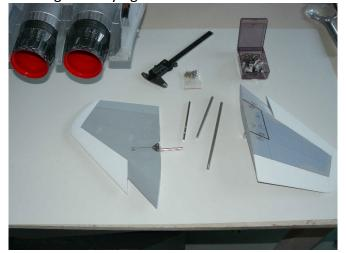
While working on the elevators, adding a small amount of lead to the inside of the LE for balance I discovered a serious problem by incorrect size of the control axles which had too much free play when fully assembled. For a one thousand dollar model I would have expected much better. New elevator axles were machined by trial and error for a perfect fit inside the installed tubes and stiffer linkages were used to eliminate any play. Secure
