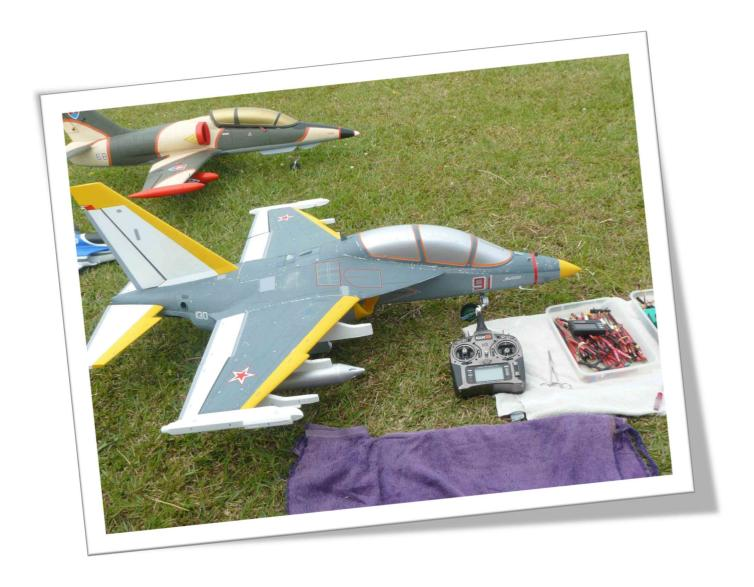
Joseph Frost's latest heavily modified YAK-130. Power is a Stumax 89 mm ducted fan rotated by a 1400 kv. Neu motor on 8S LiPos. Read the full story on Page 11.
