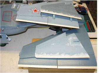
There were lot of other modifications done including thin trailing edges on all control surfaces, air intake improvements and general strenghtening of the model and the landing gear. At 4.5 kilo AUW it is rather a heavy model for a foamy and with the very scale looking landing gear and all the sequencing gear doors I knew strait away it would take all my skills to land this one!
