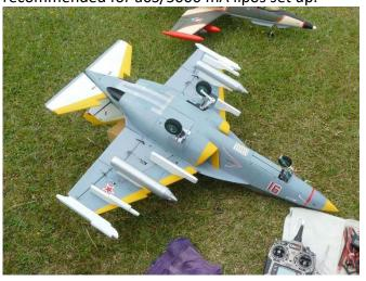
Not good enough for me, after being used to flying mainly 8S to 12S power set ups in my 90 mm EDF fleet so the first thing was testing 5 different power units to get the best out of the model. I finally decided to award the power contract to a Stumax 89 mm fan with a 1400 kv. Neu motor on 8S, about the same current draw as the recommended setup with much better power output and at only a slight increase in all up weight.
