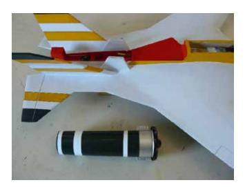
This time fitted with the large 4250mA, 25 volt battery the CofG was still spot on and after the static run while holding model vertically, it just about held its AUW at 2400grams confirming this thing will fly. Couldn't wait for the next session to test it, intending to do it again at the beach on smooth, hard-packed sand rather than off the bumpy grass where you can get premature hops with light wing loaded models.
